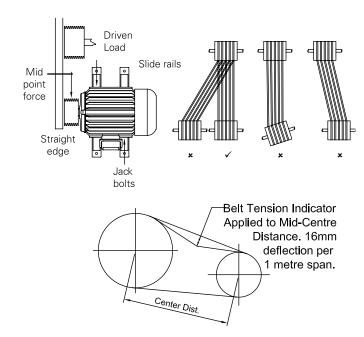
As a general rule the mid point of the applied force should be at the mid point of the shaft and it is good practice to mount the motor pulley with hub and locking screw at the
