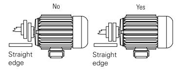
Excessive angular displacement must also be prevented. The recommended method to achieve correct angular alignment is shown below.
