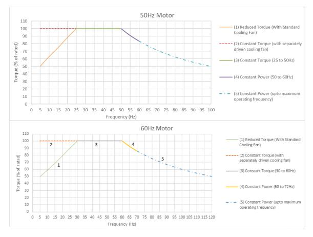
Refer to motor nameplate data for suitability on VFD supply, speed & torque range. Regal recommends use of dv/dt or sinusoidal filters when motors are operated on a VFD.
