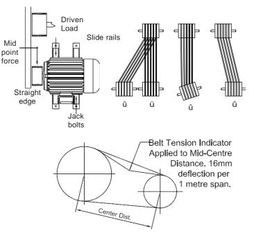
As a general rule the midpoint of the applied force should be at the midpoint of the shaft and it is good engineering practice to mount the motor pulley with hub and locking screw at the shaft end.
